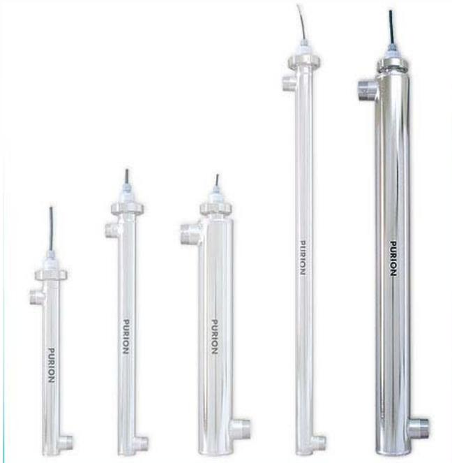
UV Plant PURION 2501 is equipped with a polished stainless steel reactor. PURION 2501 can be used to disinfect pool water up to a Volume of 50.000 l and for a transmission of at least 90% per cm. To ensure the required transmission a preliminary filter could be necessary. Other applications are fish ponds up to a volume of 30.000 l at continuous recirculation.
