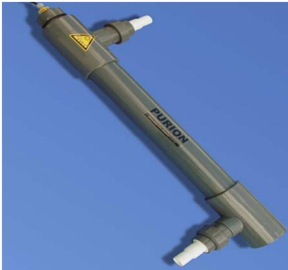
UV Plant PURION 2501 PVC is equipped with a PVC-U reactor. PURION 2501 PVC-U can be used to disinfect pool water up to a Volume of 50.000 l and for a transmission of at least 90% per cm. To ensure the required transmission a preliminary filter could be necessary. Other applications are fish ponds up to a volume of 50.000 l at continuous recirculation.
