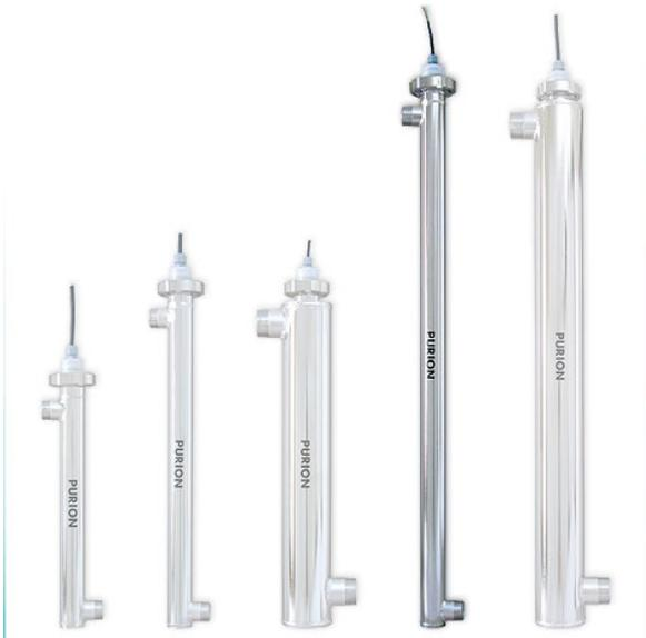
UV Plant PURION 2500 H is equipped with a polished stainless steel reactor. PURION 2500 H can be used to disinfect high temperature water especially to protect legionella. It's possible to disinfect drinking water up to a flow rate of 4.000 l/h and a transmission of at least 90% per cm.
