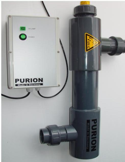
UV Plant PURION 2001 PVC is equipped with a PVC-U reactor. PURION 2001 PVC-U can be used to disinfect pool water up to a Volume of 30.000 l and for a transmission of at least 90% per cm. To ensure the required transmission a preliminary filter could be necessary. Other applications are fish ponds up to a volume of 30.000 l at continuous recirculation.
