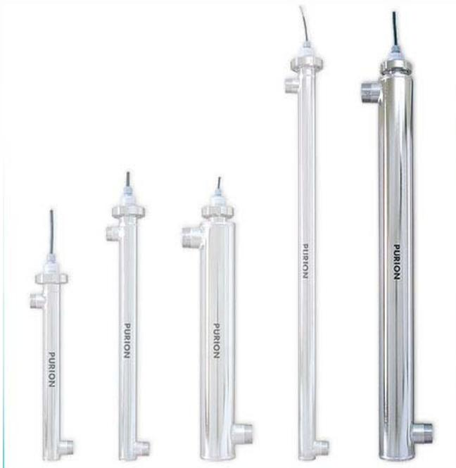
UV Plant PURION 2501 H is equipped with a polished stainless steel reactor. PURION 2501 H can be used to disinfect high temperature water especially to protect pool water against legionella. It's possible to disinfect pool water up to a volume of 50.000 l and for a transmission of at least 90% per cm.
